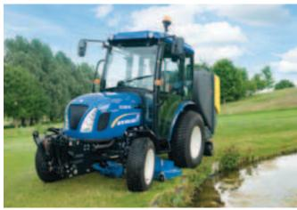
Class 3. Boomer 40 and Boomer 50 Four-cylinder 41hp(CV) and 47hp(CV) engines, three-range hydrostatic or 16x16 synchromesh transmission
