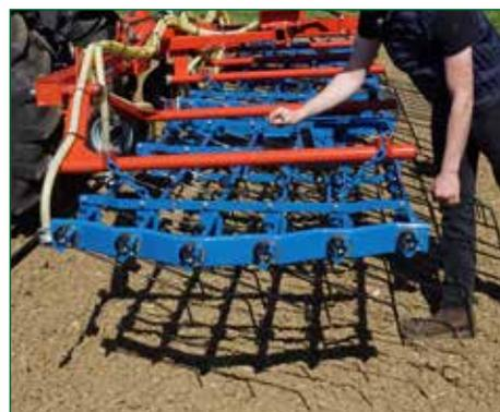
Ground conditions will determine how aggressive the tine pressure needs to be for effective harrowing.
