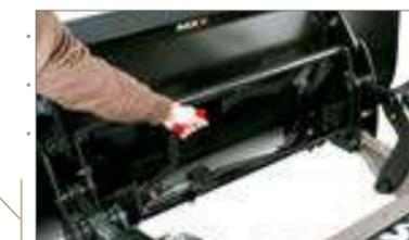
Automatic locking implement carrier. Externally accessible release handle.
