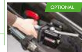
Instant multi-coupling for loader/implement hydraulics with the MACH 2® connector. [page 50](#)
