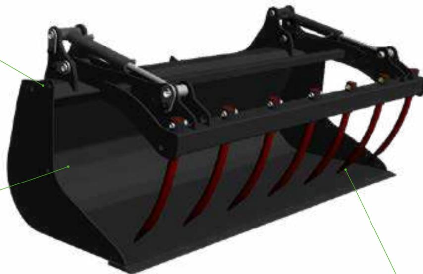
Tines set back from the blade to pick up material right down to the foot of the wall
