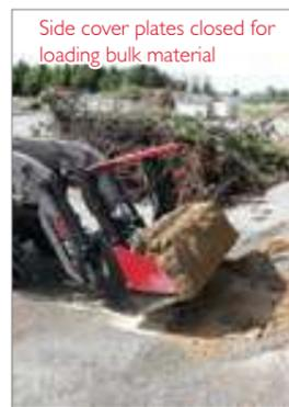
Side cover plates closed for loading bulk material
