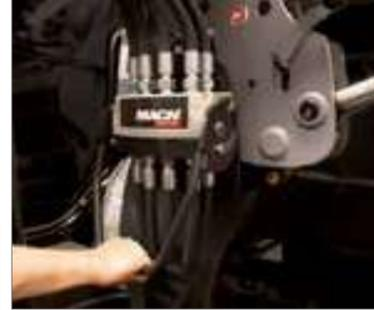
MACH System® – sealed instant coupling of tractor to loader hydraulic and electric lines. [▶ page 50](#)
