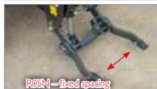
Depending on the tractor, a linkage with fixed spacing (R05N/R08N) may be possible.
