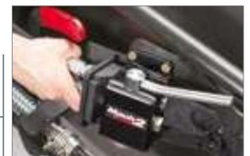
Instant multi-coupling for loader/ implement hydraulics with the MACH 2® connector.
