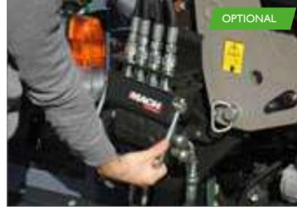
**MACH System®** – “non drip” instant coupling of tractor to loader hydraulic and electric lines \* [page 50](#)
