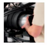
The engine air filter is easy to check, clean or replace, with no need for tools.
