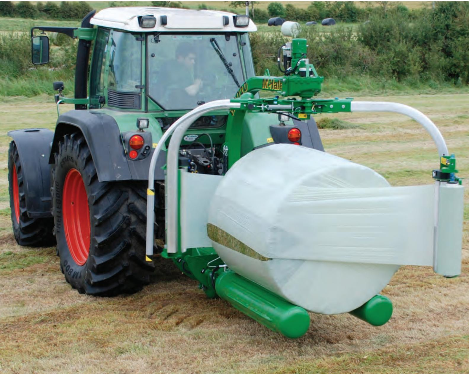
**T**he McHale W2020 is a high-speed stacking bale wrapper. It is a compact machine, which allows one operator to transport, wrap and stack the bale with one tractor or loader. The W2020 can wrap a bale with four layers of plastic in approximately 20 seconds and with six layers of plastic in 30 seconds. The W2020 is controlled by an expert plus control box, which makes wrapper operation fully automatic.
