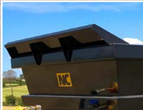
Weld on Stone Guard
