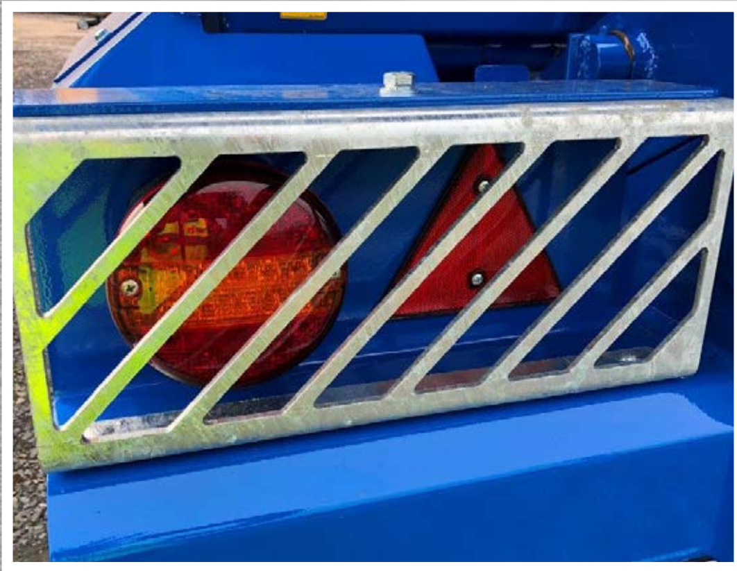
LED Lights and Galvanised Guards
