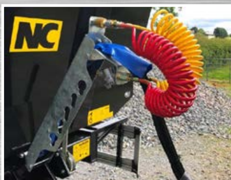
Air & Hydraulic Brakes or Air Only Brakes
