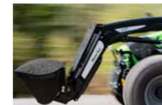
DRIVE SMOOTHER WITH SOFTDRIVE SoftDrive® is a loader suspension system that will improve your everyday loader work. With SoftDrive® protecting everything between the load in the implement and the ground you can work more efficiently. SoftDrive® not only reduces the stress on the loader and the attachment but also the tractor, the tires and even you as the driver.
