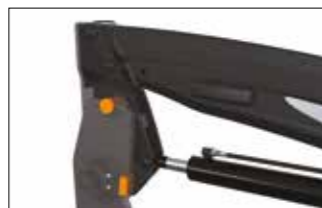
SUPER STRONG SUBFRAME Quicke's Delta subframe has oversized dimensions with precision machined contact surfaces. The wide U-support and large locking pin enables the loader to cope with difficult and heavy jobs for many years.
