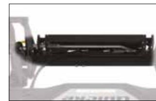
Q-LOCK – HYDRAULIC IMPLEMENT LOCKING Our improved hydraulic implement locking ensures simple and comfortable changes of implements. Unlock, change implement and lock without getting out of your drivers seat.
