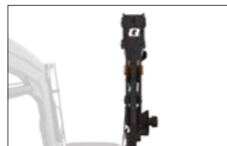
OPTIMAL DIVISION OF POWER The compact and profile-pressed bearing box is narrow close to the locking pin. This means that the locking pin can be made short and strong, while the wide U-support provides maximum stability with heavy loader jobs.
