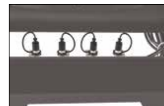
4TH FUNCTION This option provides hydraulic power for implements requiring 2 separate double-acting functions. 4th function requires 3rd function to be installed and the couplings are neatly fitted adjacent to the 3rd function couplings.
