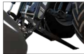
ROCK-STEADY SUPPORT LEGS Fully integrated heavy-duty design with flexible positions makes it quick and easy to connect and disconnect your Quicke® loader. No tools are required and there are no loose parts.
