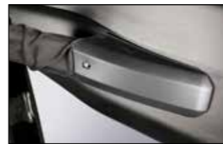
SMART OUTLET The hose routing inside the loader beam comes out well protected on the side of the loader. Good for visibility and good for protection of hoses.
