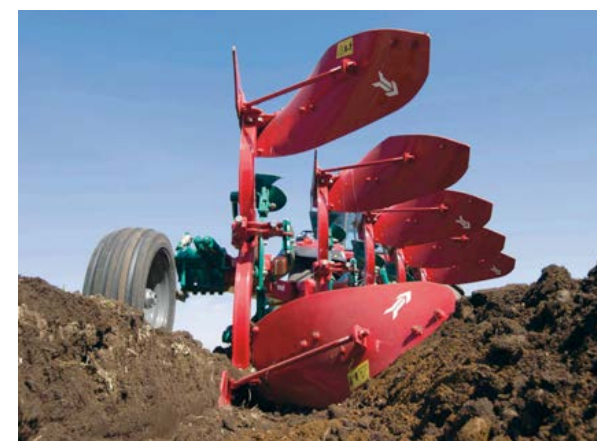
furrow profile body No. 28 working depth: 26 cm, bottom: 30 cm, width 73 cm
