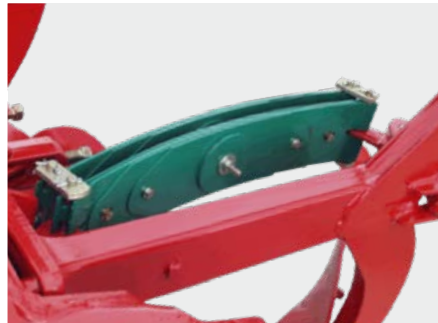
Double spring package with 14 leaves (1400 kp)
