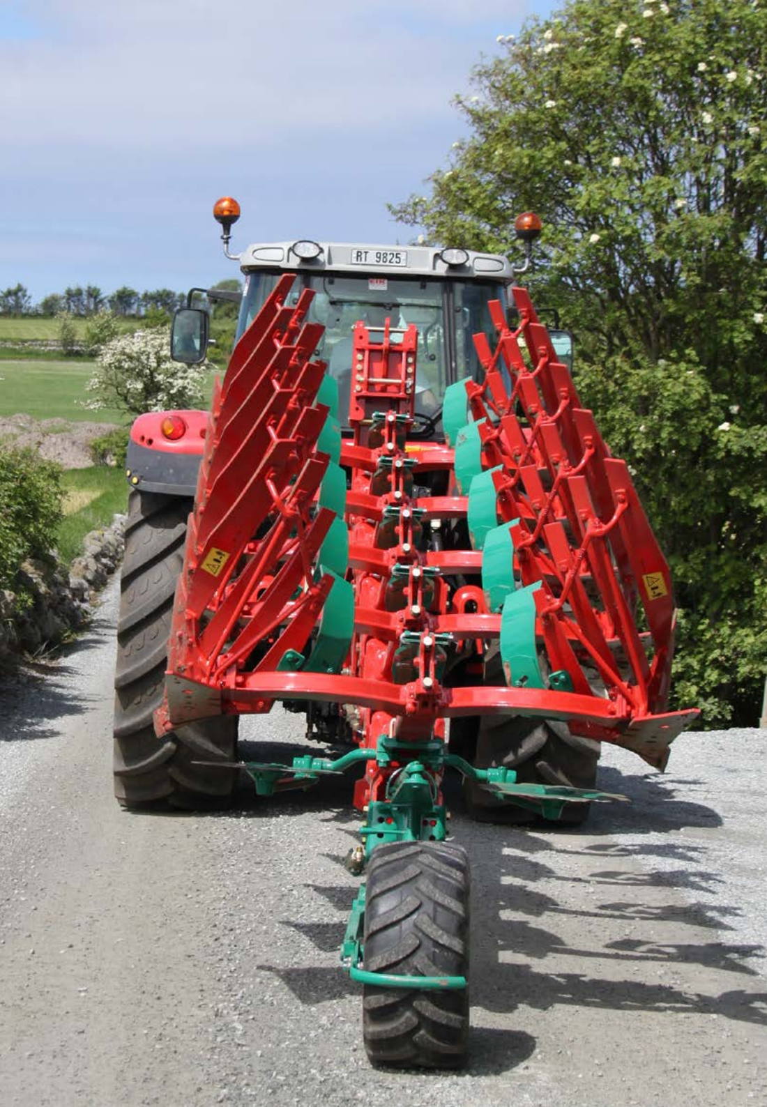
Transport position. Rear mounted depth and transport wheel
