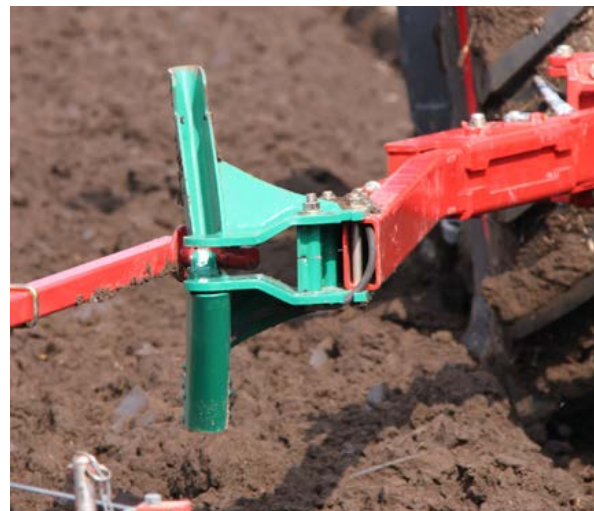
Packer arm connecting to the packer
