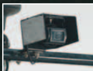
A rear mounted viewing camera enables operators to view bale delivery and to monitor bale accumulator performance in real time. Mounted on the rear rail, footage is displayed on the IntelliView™ monitor. Operators can choose full screen or split screen viewing when the top of the range IntelliView™ IV display is fitted.
