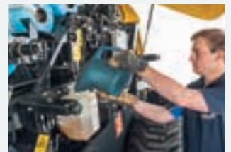
Chains lubricated with universal 10-40 oil. Chain oiling brushes operate each time the baler tailgate is opened.
