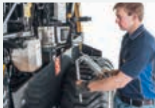
Lincoln centralised lubricating system is easy to check and simple to fill.
