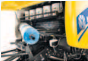
Integrated prop to support a roll of net when changing it from ground level.
