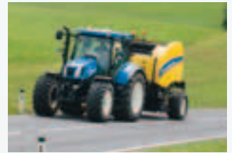
Optional ultra-wide 500/55-R20 tyres reduce compaction to facilitate regrowth for subsequent silage cuts. They also deliver more comfortable road transport.
