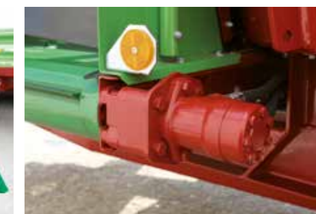
Hydraulic motors – depending on the application, you can select from a range of motors of different speeds.
